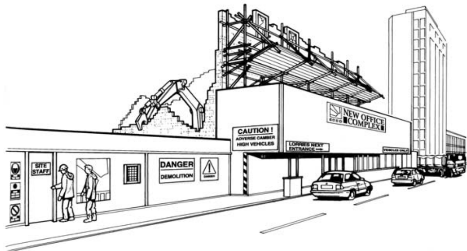
Figure 3 Office demolition in a city centre showing separate entrances for workers and vehicles and a protected thoroughfare
