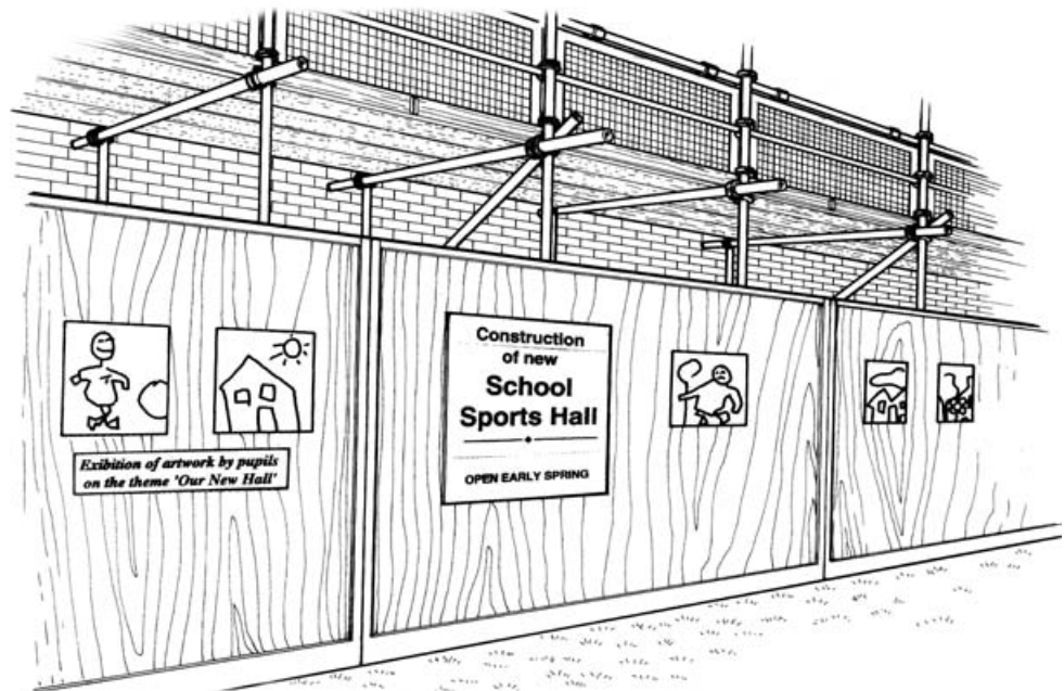
Figure 4 Panels are fixed around the base of the scaffolding to prevent children from climbing
